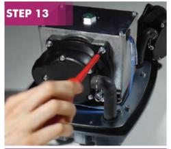
Connect the chamber block and diaphragm together and screw back into place. Repeat on the opposite side of the pump.
