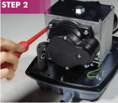
Unscrew the chamber cover at one end of the pump. Separate the chamber cover at the seam to expose the screw holding the white round plastic diaphragm depressor in place.
