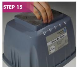
Remove the dirty filter and clean away any dust or dirt that has been collected.
