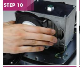
Remove the diaphragm frame and peel off the worn diaphragm.
