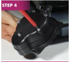
Unscrew the chamber block and pull it apart.
