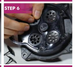
Pull the new valves through, you should hear a 'snap' sound once secured in place.
