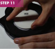
Replace the worn diaphragm with the new one provided in your service kit. Make sure the diaphragm has been pushed into the grooves of the diaphragm frame. Repeat this process on the opposite side of the pump.
