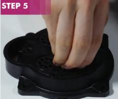
Remove the valves from the chamber block, take note of the valve formation.
