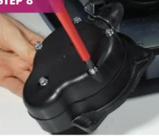
Screw the chamber block back together ensuring the rubber seal between them lined up properly. Repeat this process on the opposite side of the pump.
