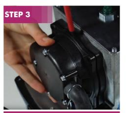
Unclip the diaphragm face to expose the diaphragm and chamber block.
