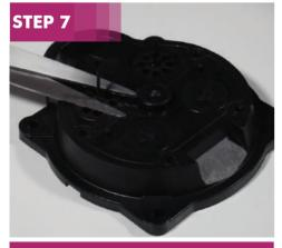
Cut the excess rubber off from the valves and discard.
