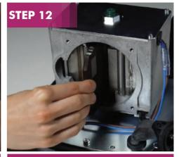
Remove the worn magnet and replace with the new one provided.
