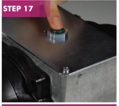
Note: Before screwing the pump back together ensure the safety switch button is pushed down. If this step is not completed then the pump will not run.
